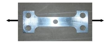
Fig. 2. Aluminium Test Specime.
